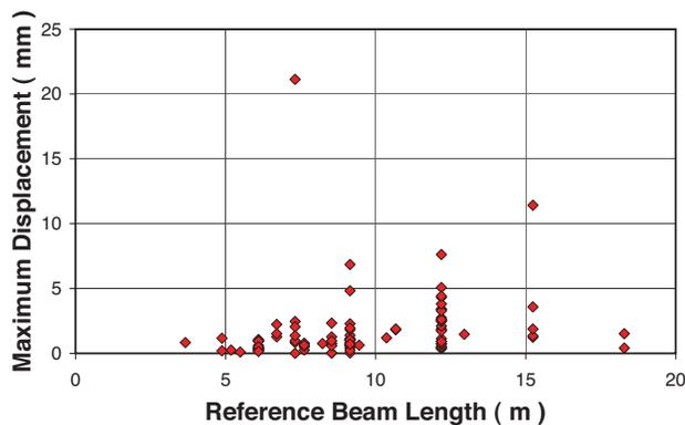
[FIG. 2] Maximum Reference Beam Displacement vs. Beam Length (LOADTEST Database, 1995-2004)
